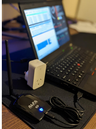
Figure 3: Equipment used (from left to right) an Alfa AWUS036NHA, the Kasa Smart Plug KP115 and Linux ThinkPad
